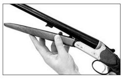
Attach the stock first to the receiver and then to the barrel properly and then press it strongly.
